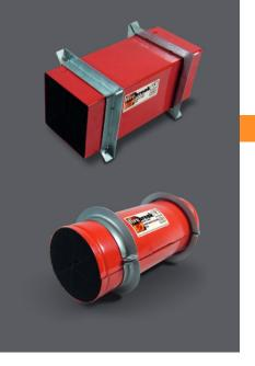
Firebreak Service Transits comprise a range of circular and rectangular devices designed to be installed in fire resistant walls and floors where cables and other services are required to penetrate. Under fire conditions the foam plugs at each face of the transit restrict the passage of smoke whilst the intumescent material within the transit expands to form a durable plug around the services maintaining the fire integrity and insulation performance of the floor or wall.
