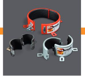
Firebreak FX400 Pipe Collars comprise a range of devices primarily designed to be fitted around plastic pipes where they penetrate fire separating constructions. Under fire conditions the intumescent material within the collar expands to crush the softening pipe and fill the resultant opening, thereby maintaining the fire integrity and insulation performance of the floor or wall.
