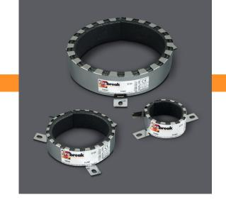
Firebreak FX300 Pipe Collars comprise of a range of devices designed to be fitted around plastic pipes or insulated metal and plastic pipes where they penetrate fire separating constructions. Under fire conditions the intumescent material within the collar expands to crush the softening pipe and/or combustible insulation, filling the resultant opening and maintaining the fire integrity and insulation performance of the floor or wall.
