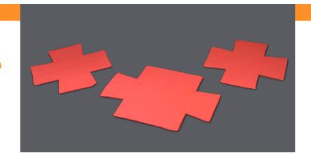
Firebreak Electrical Box Protectors (Putty Pads) are designed to reinstate the fire resistance of partitions when fitted with electrical socket and switch boxes. Made from silicone-based intumescent polymer with additional fire resistant additives they are non-setting and mouldable for quick and easy installation.
