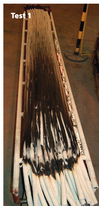
Limited damage to cables after test
