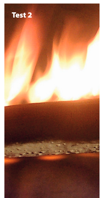
High voltage cable exposed to 700°C flame
