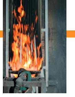
Firebreak C100 Cable Coating is a durable fire resistant water-borne coating designed for application to conventional cable installations. In the event of a fire it prevents flame spread along both horizontal and vertical cable runs and can also be used to maintain the circuit integrity of critical power and control cables for up to 2 hours.
