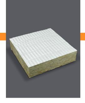
Firebreak Batts are stone mineral wool boards coated on both faces with a flexible fire resistant ablative coating. They are used to form fire and smoke stop seals able to reinstate the fire resistance of separating walls and floors when penetrated by a wide range of building services.
