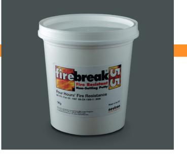
Firebreak 55 Fire Resistant Non-Setting Putty is designed to reinstate the fire resistance of small cable and metallic pipe service penetrations through walls. Made from silicone based ablative polymer with additional fire resistant additives it is non-setting and mouldable for quick and easy installation by hand. If required, the putty can be removed to allow changes to the penetrating services and then re-used to reinstate the fire seal.
