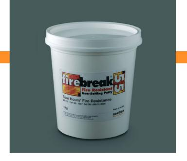
Firebreak 55 Fire Resistant Non-Setting Putty is designed to reinstate the fire resistance of small cable and metallic pipe service penetrations through walls. Made from silicone based ablative polymer with additional fire resistant additives it is non-setting and mouldable for quick and easy installation by hand. If required, the putty can be removed to allow changes to the penetrating services and then re-used to reinstate the fire seal.
