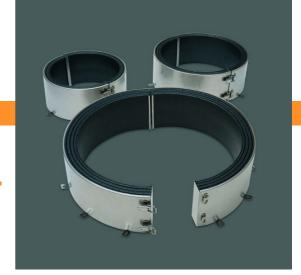
Firebreak FX500 Pipe Collars comprise of a range of devices primarily designed to be fitted around large plastic pipes where they penetrate fire separating constructions. Under fire conditions the intumescent material within the collar expands to crush the softening pipe and fill the resultant opening, thereby maintaining the fire integrity and insulation performance of the floor or wall.
