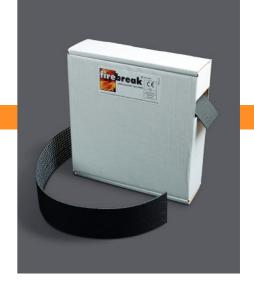
Firebreak FX200 Sealstrip is a durable intumescent strip material supplied as a continuous 10m roll packed in a convenient self-dispensing box to be cut to length on site as required. It is designed to be installed around plastic pipes or metal pipes with combustible insulation where such services penetrate fire resistant walls or floors providing fire seals of up to 240 minutes.
