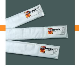
Firebreak FX200 Pipe Wraps comprise a range of different sized plastic sleeves containing one or more layers of durable intumescent strip material pre-cut to suit a wide range of different pipe sizes. They are designed to be installed around plastic pipes or metal pipes with combustible insulation where such services penetrate fire resistant wall or floors providing fire seals of up to 240 minutes.
